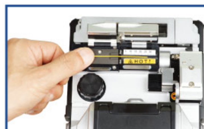
Stripping (No Cracks on Fiber)
